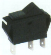
FC-H-0147 (ASW-09-101,ASW-09-102) ASW-09-101:ON-OFF SPST 2P ASW-09-102:ON-ON SPDT 3P 20A 12VDC;10A 125VAC
