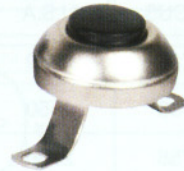
FC-H-0145 (ASW-08H) OFF-(ON) 3A 30VDC; 6A 12VDC SPST 2P
