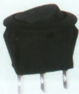
FC-H-0165 (RS-101-8C,RS-102-8C,RS-103-8C) RS-101-8C:ON-OFF 2P RS-102-8C:ON-ON 3P RS-103-8C:ON-OFF-ON 3P 20A12VDC;10A125VAC
